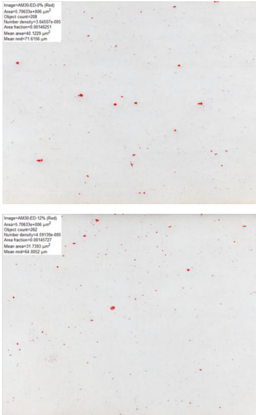
Figure 2.1 Optical Micrographs with image analyses of the AM30 alloy at (a) the initial state, 0%, and (b) after 12% of true strain. It was concluded from these optical analysis results that the area fraction particles remained constant from during tensile testing, with almost no voids nucleating on them.
